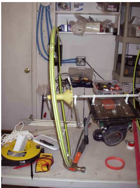
The bent left wheel after test 71
