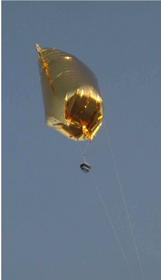
The balloon and payload attachment in the same configuration as in the morning EVA but with a mini DV camera as payload.
