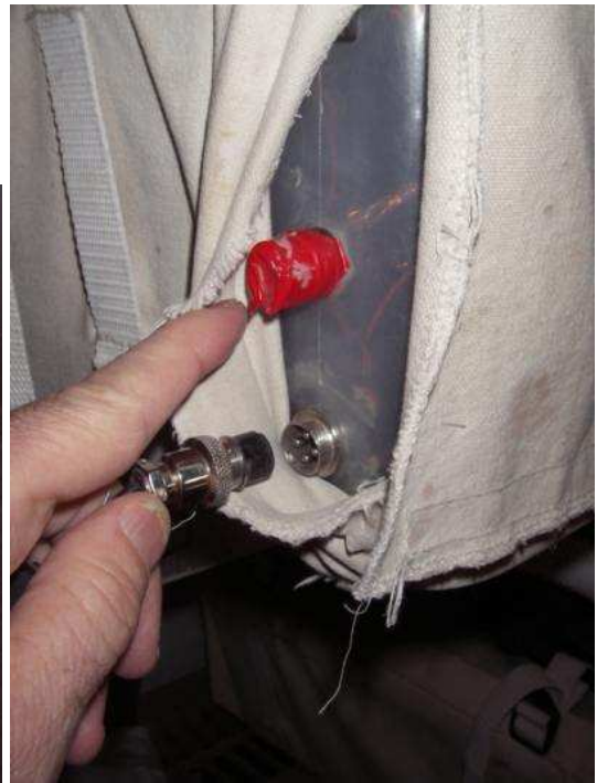
The battery loading connector and fuse location in red.
