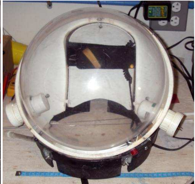
Helmet front view. The “push to talk” is on the lower right (it is red on this helmet). The two clamps interfaces are visible in the lower collar. Right and left the air inlets are equipped with laterally oriented injectors. The black horizontal band in the upper part is the fixation of the radio bag. The wire connecting the radio to the microphone and the “push to talk” button is visible on the right.
