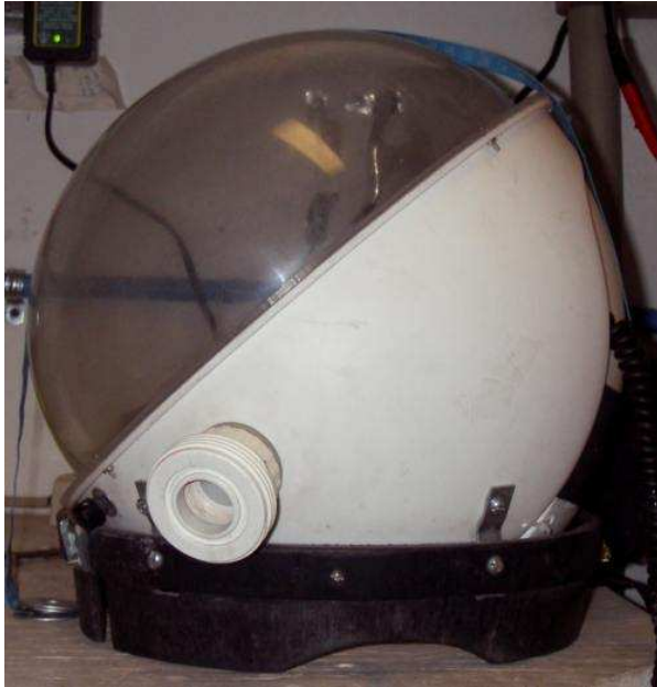
Helmet lateral view. The “push to talk” button is in the lower left, left of one of the air inlet interfaces.
