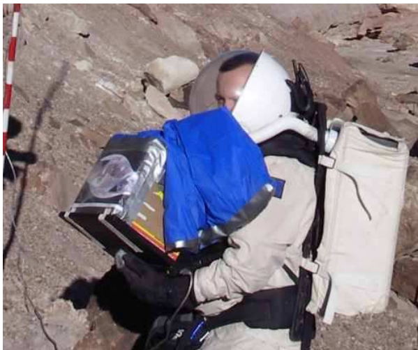
The sun screen box used to observe the laptop screen during the pole mounted camera operations
