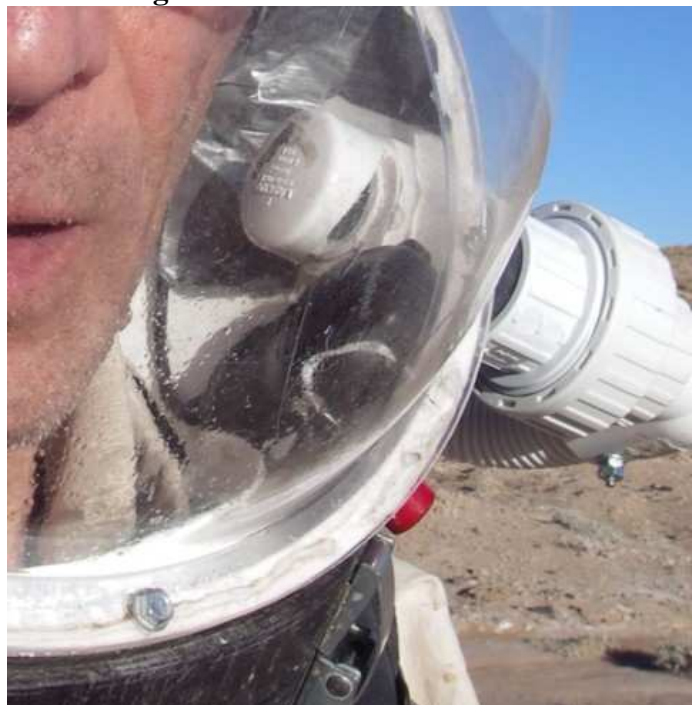
Photo taken during EVA 17 showing the microphone, the red “push to talk” button and the laterally oriented air injection. Some droplets of water are condensed in the lower helmet visor which has no consequences on the visibility.
