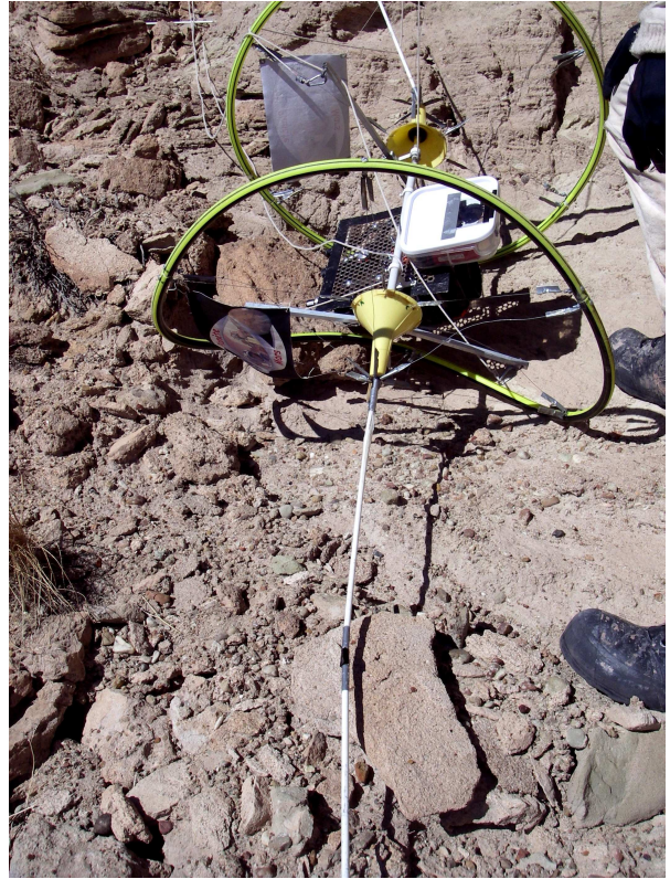
Stacy's Cake: a very difficult cliff for the CRV. On the left the vehicle is still under control. On the right the vehicle as found by the retrieval team. The right wheel is deformed, the anti roll rods are bent.
