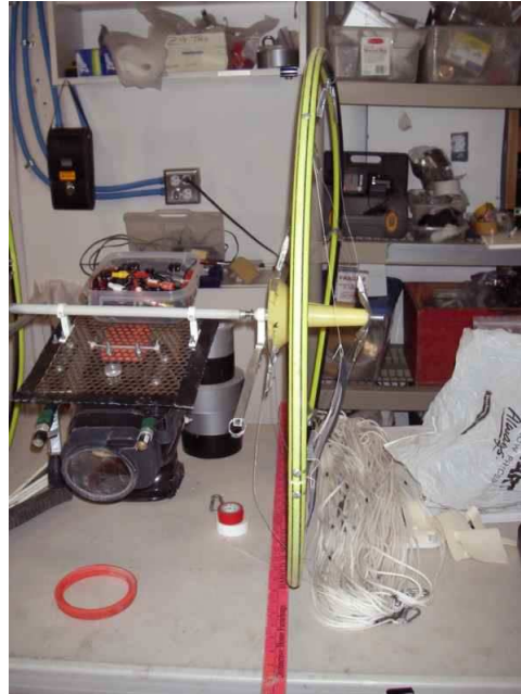
The bent right wheel after test 71
