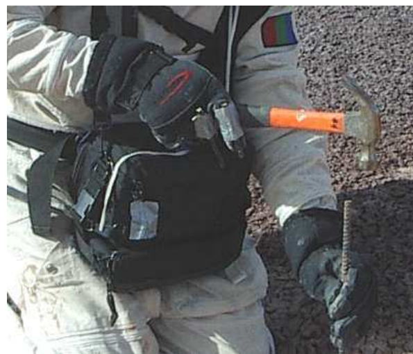
The belly camera bag and the zipper grip enlarged with a 5X6 cm tape to facilitate the opening and closing (EVA 11). The right glove is in configuration A2.
