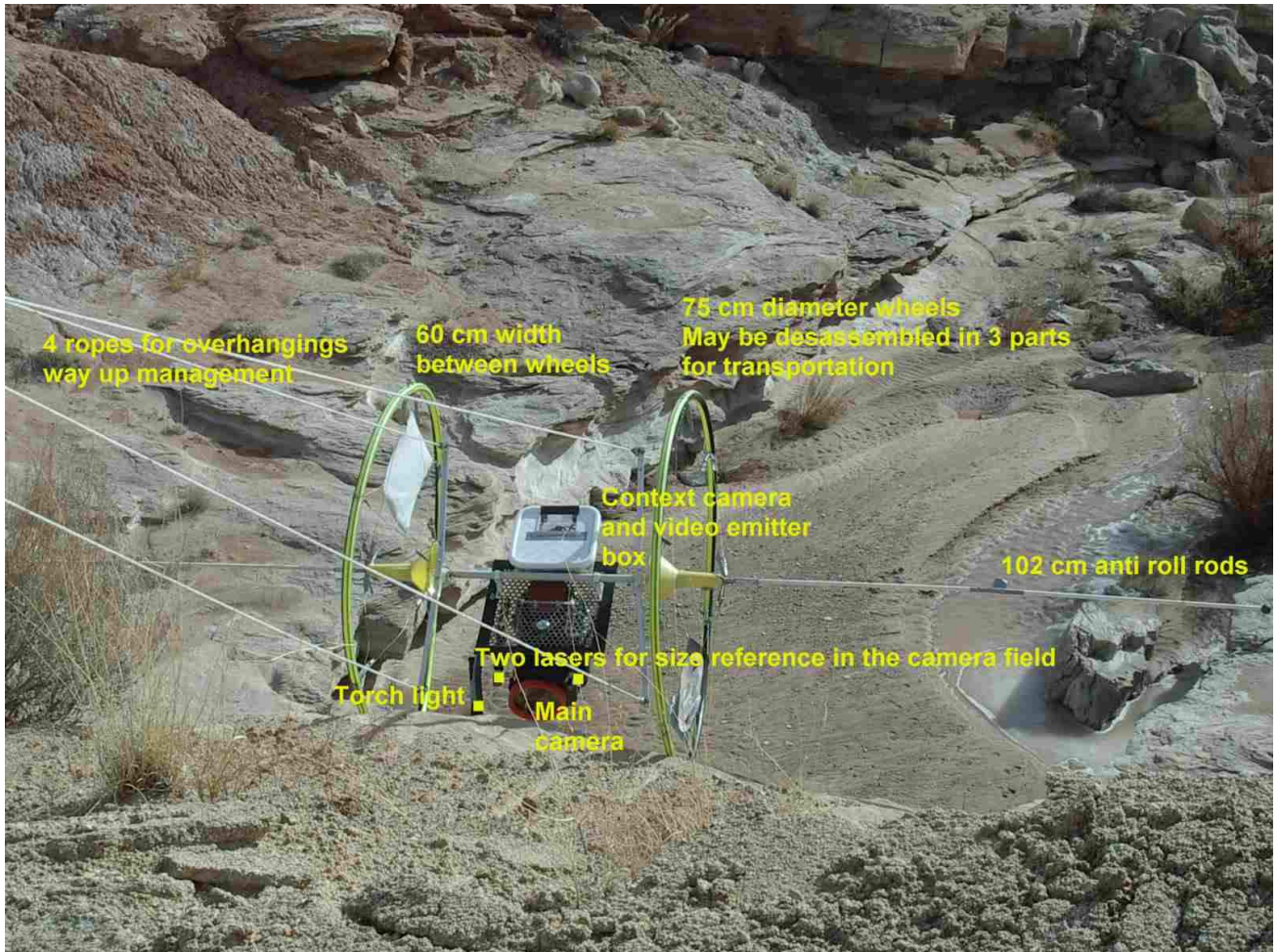
Cliff Reconnaissance Vehicle n°3 main features (CRV test 70 at White Rock Canyon).
