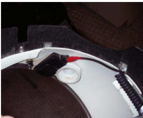
A view from under showing the microphone inside the helmet.
