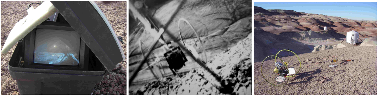
The picture received up the hill (left) from the context camera and recorded (middle) on the hard drive. The X cross is the grid protecting the camera lens. On the right the CRV and 1.3m on its right the context camera yellow container.
