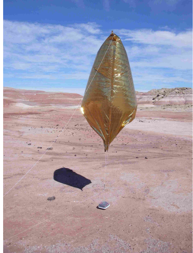
The balloon and the CRV box as payload On the left the two ropes, one linked to the upper part, the other to the payload support lines. The balloon is slightly deflated.
